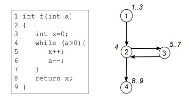
Figure 2.11: CFG for Iteration (while)
