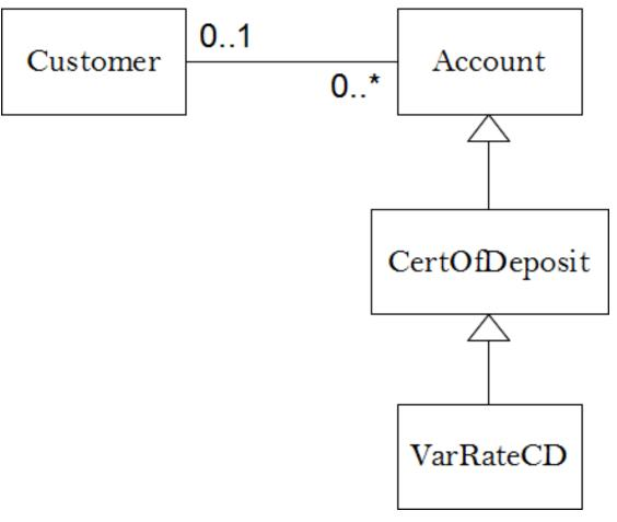
Figure 6.3: Class Diagram for Banking System
