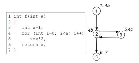
Figure 2.13: CFG for Iteration (for)
