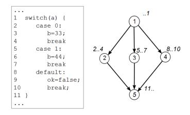
Figure 2.10: CFG for Selection (switch)
