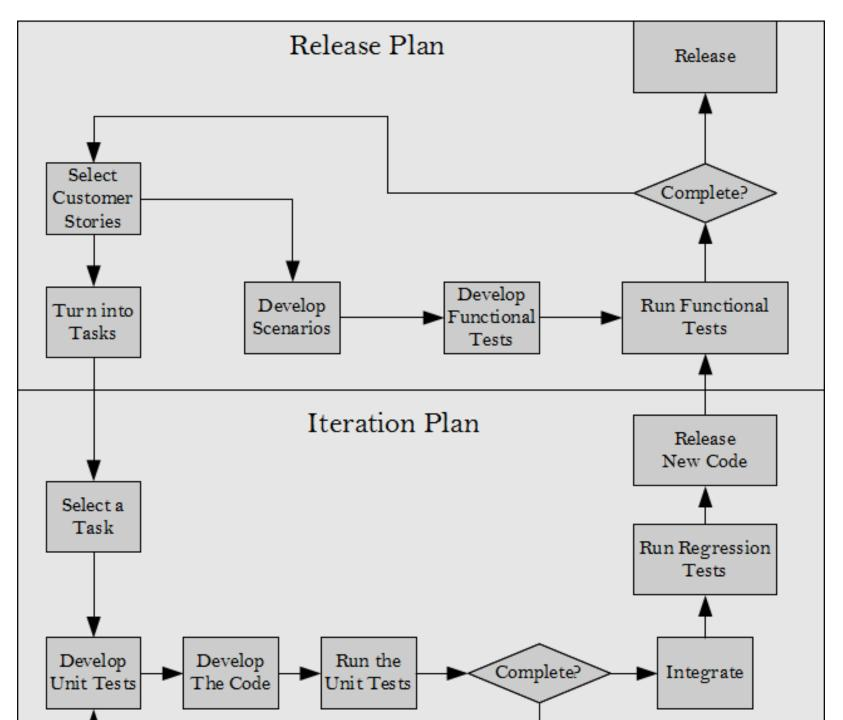
Figure 9.7 is a diagram of the XP process, highlighting the testing activities.
