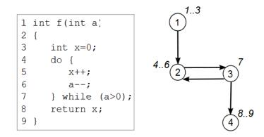
Figure 2.12: CFG for Iteration (do-while)
