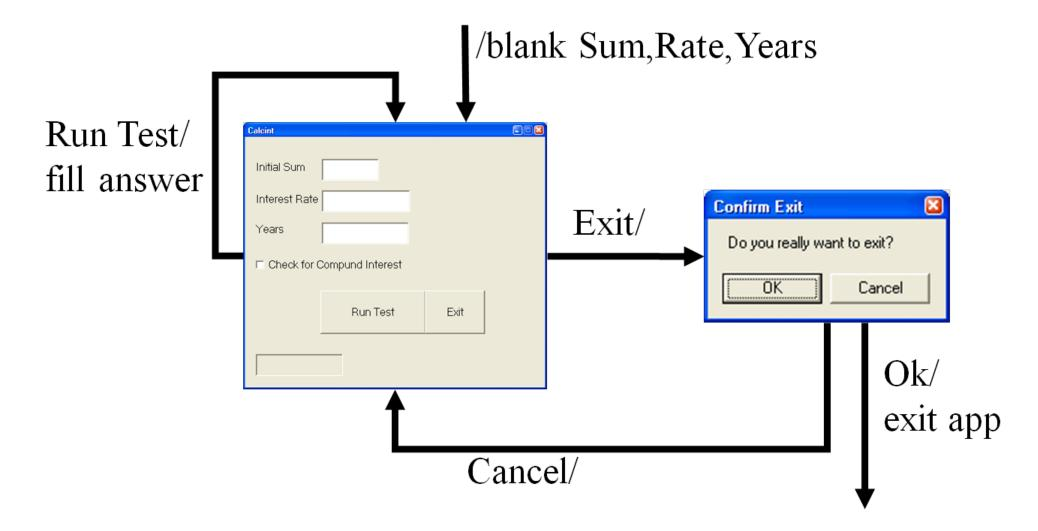
Figure 7.13: Calcint GUI State Diagram
