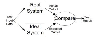
Figure 2.1: Software Tests Procedure
