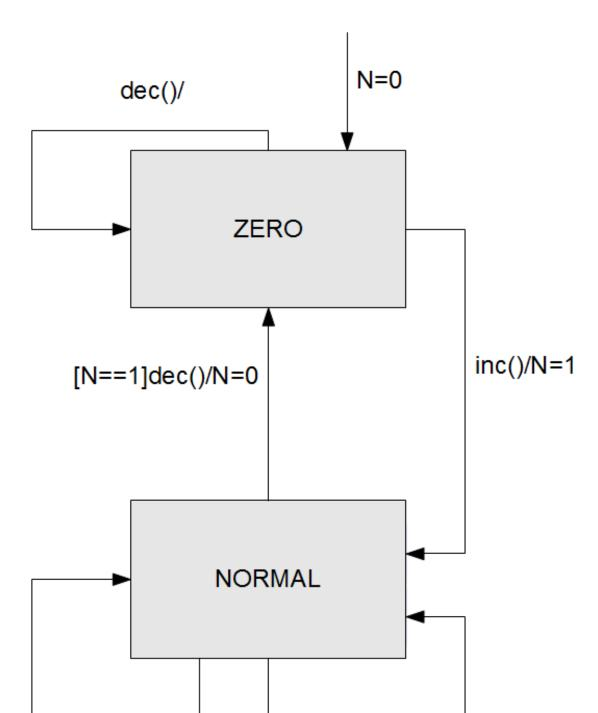
The state diagram shown in Figure 2.6 specifies the response of a counter with three defined methods: *inc*rement the counter, *dec*rement the counter, and *getValue*. The state diagram specifies that:
