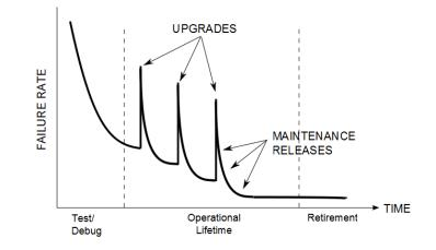
Figure 1.1: Failure Rate for a Software Product over its Lifecycle
